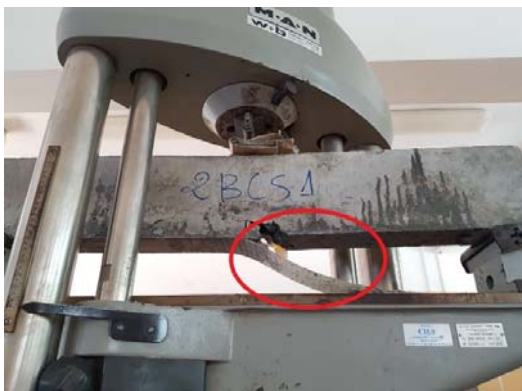
Fig.6. Peeling off GFRP sheets
