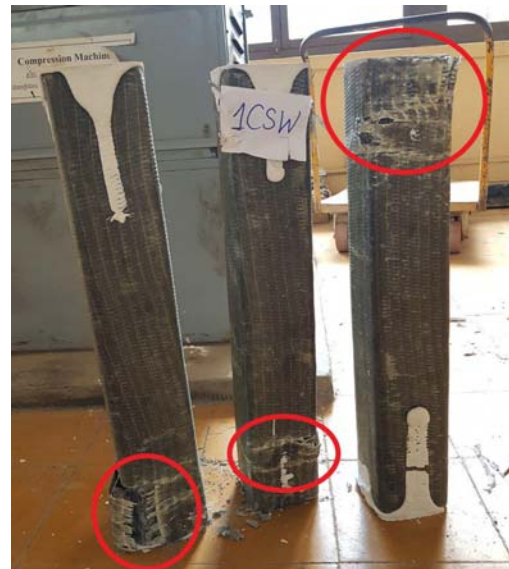
Fig.8. Rupture along direction of GFRP of strengthened column
